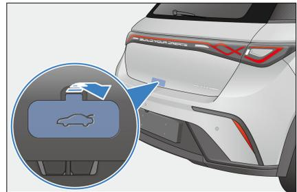
2. Pull the lever to unlock the trunk.
