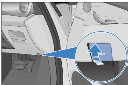
2. To open the hood: Lift up the hood and support it with the with a stay bar.
