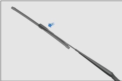
3. Hold the wiper blade and pull it out along the indicated direction.
