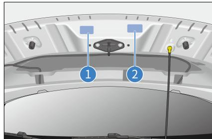
Side airbag warning labels are attached below the left and right B-pillar lock rings.
